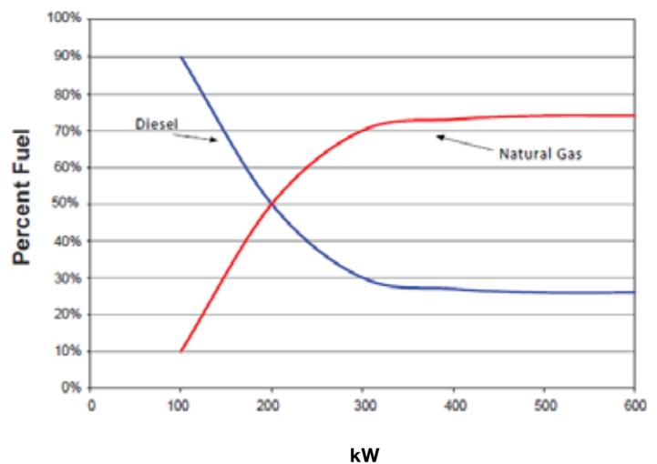
Figure 1. BiFuel % Diesel and Natural Gas
