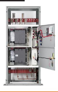
Bypass Isolation Transfer Switch 100 – 1200A, up to 600VAC, 50/60 Hz 3 or 4 poles NEMA 1 or 3R Closed Transition UL1008 Listed CSA C22.2 No. 178 Certified
