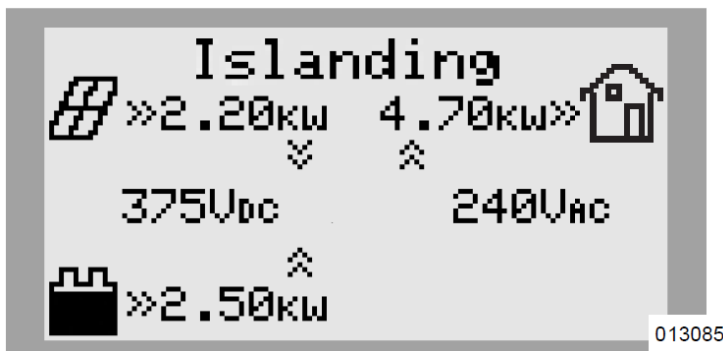
Figure 4. Island Mode with the Generator Inhibited.
