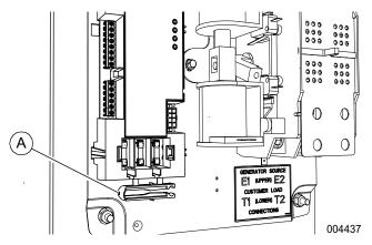
Figure 4-2. Fuse Removal and Installation Tool
