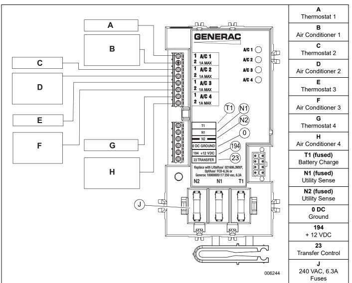
Figure 3-3. Typical SACM Connections
