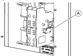
Figure 3-4. Auxiliary Contact
