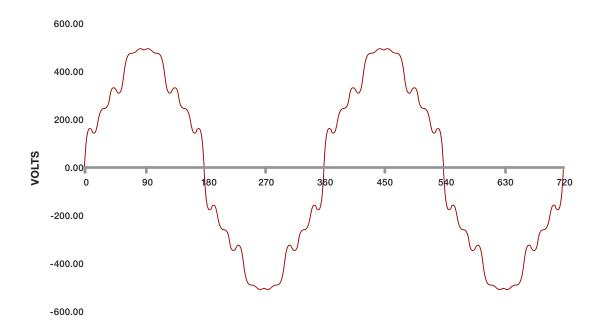
Total Harmonic Distortion (THD) can affect the generator due to harmonic currents produced, which in turn flow through the alternator, taking up capacity and creating heat. Two ways to address this is to utilize filtering devices or reduce the source impedance by upsizing the alternator or adding other loads.
